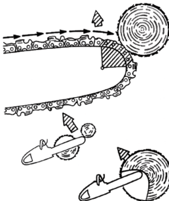
Figure 2. Kickback occurs when the tip of the chainsaw comes in contact with a solid object at the wrong angle.
